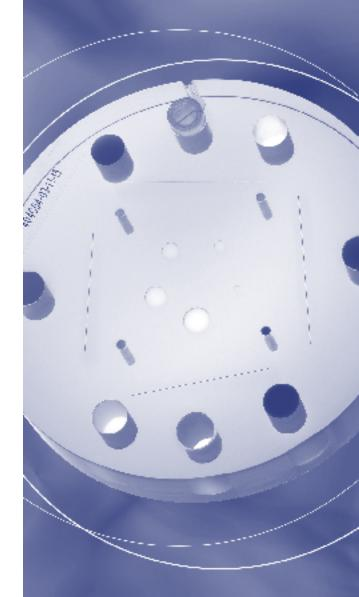
Two sets of opposing wire ramps aligned with the x and y axes are cast into the CTP401/404 module. These ramps are used to measure scan slice geometry, verify phantom position and check the patient alignment system and the scanner table incrementation.
